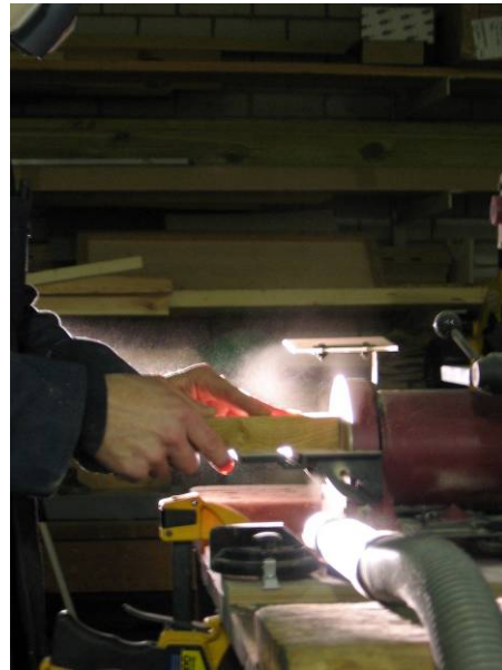
Figure 5b. The same sanding process using the dust-lamp
