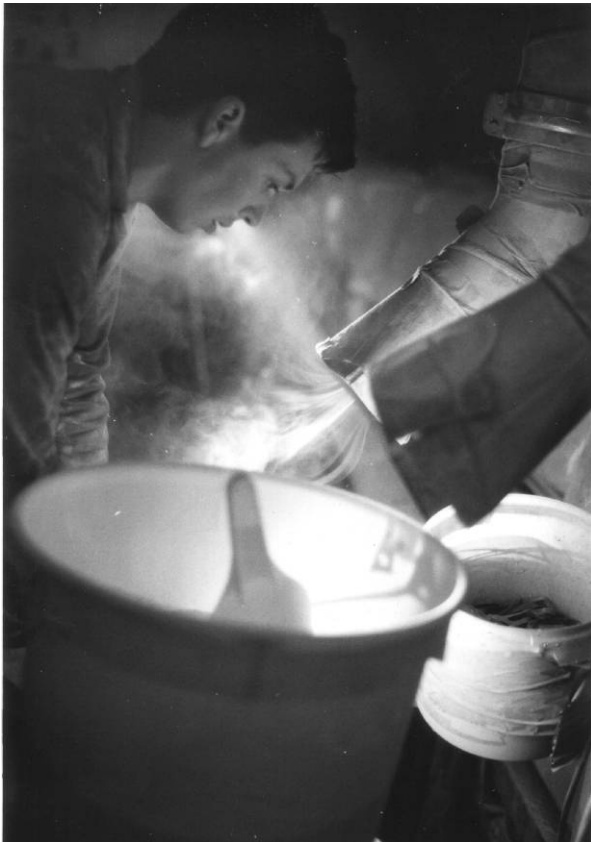
Figure 6 A dust-lamp shows a small capturing LEV hood ineffectively controlling dust exposure
